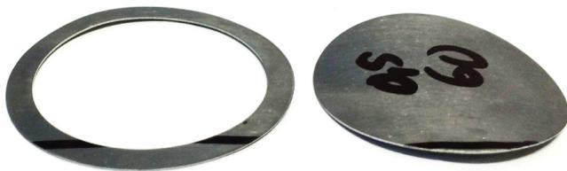
Figure 7 Rotary cut toroidal laminations
